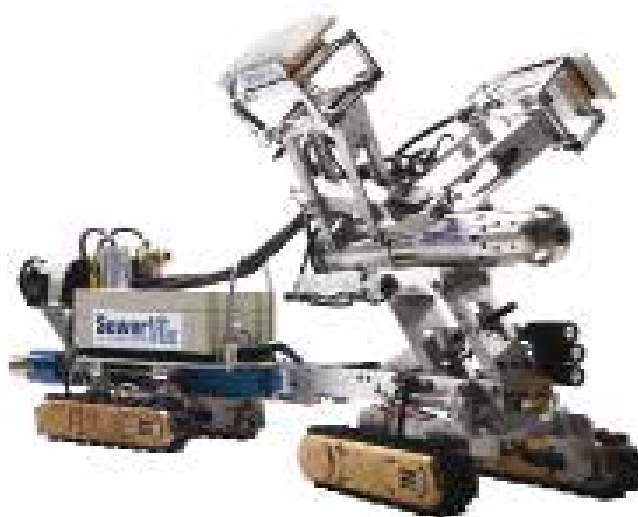
The SewerVUE Surveyor is the first commercially-available inspection robot to use CCTV, LIDAR and PPR to inspect underground pipes.
