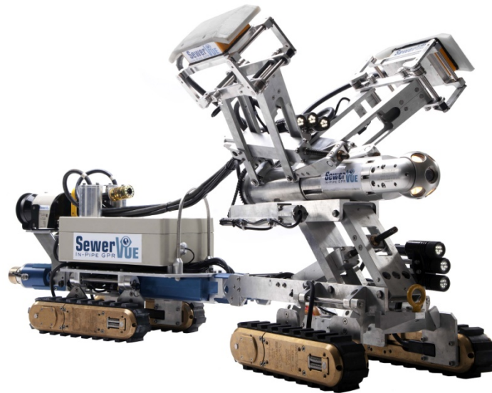
Figure 1. Fourth generation multi-sensor inspection robot equipped with pan, tilt, zoom CCTV, LIDAR, and pipe penetrating radar.
