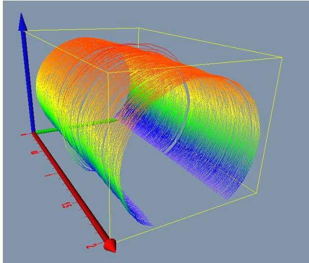
Figure 3. 3D view of a 24" plastic pipe joint generated from laser data.
