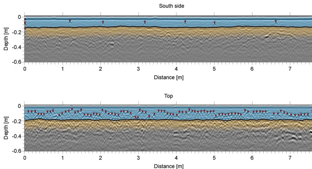
Figure 6. Interpreted PPR data from a) side wall, and b) obvert of the 30" box culvert in Port Moody, BC. Pipe wall thickness is marked by black line, rebar is represented by red dots.
