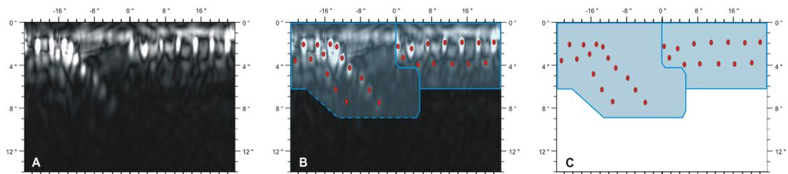
Figure 4. PPR cross section (B-Scan) showing joint configuration in a 60 inch reinforced concrete pipe. A: processed and migrated PPR data, B: processed data with interpretation overlay, C: interpretation. Red dots represent rebar. Scale in inches.
