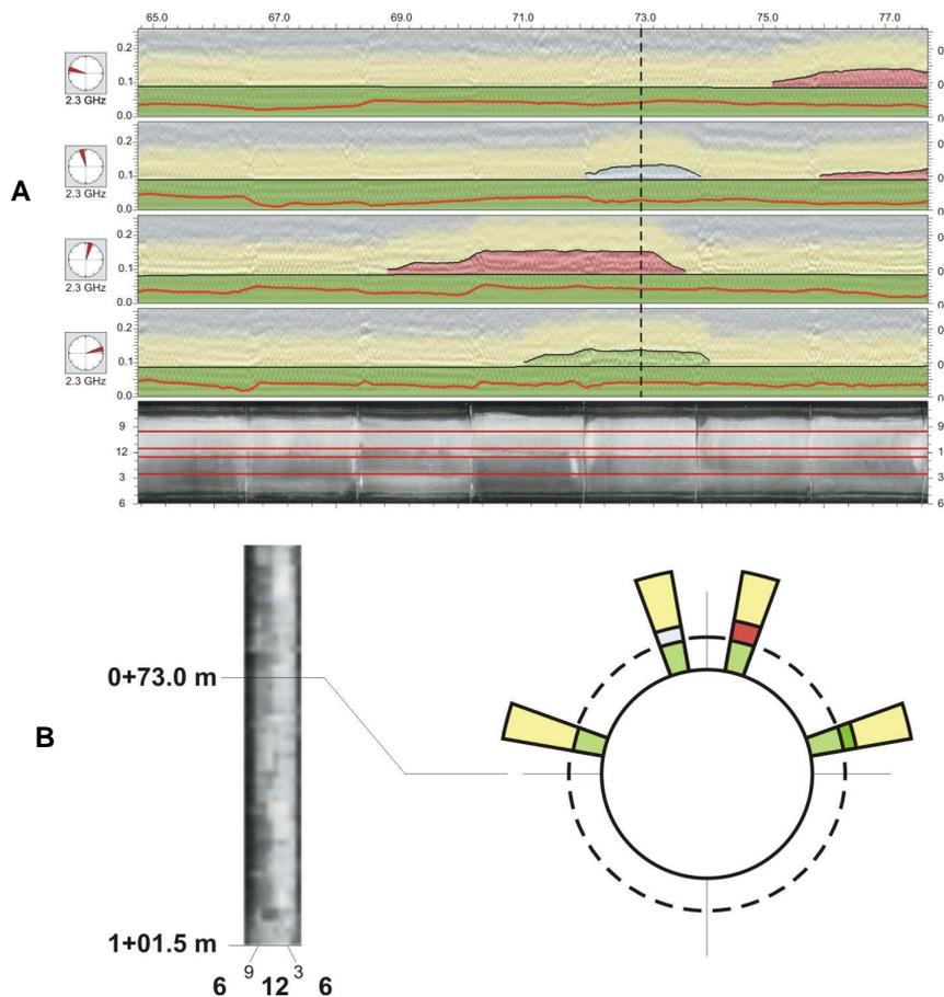
Figure 5. PP RADIAN views of a 30'' (750mm) reinforced concrete sewer pipe: A: longitudinal cross sections at multiple clock positions with corresponding CCTV foldout view. B: Cross section view with corresponding CCTV foldout view.
