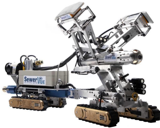
Figure 2. The fourth generation SewerVUE Surveyor multi sensor inspection robot equipped with HD pan tilt zoom CCTV, PPR and LIDAR.
