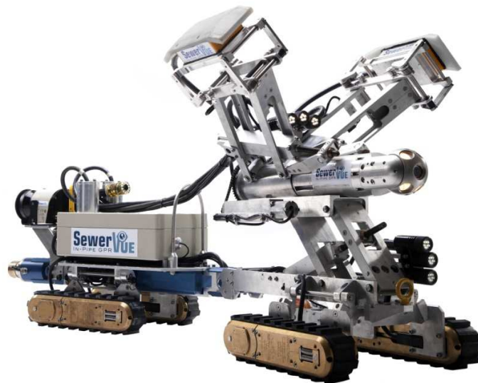
Figure 2. Fourth generation multi-sensor inspection robot equipped with pan, tilt, zoom CCTV, LIDAR, and pipe penetrating radar.
