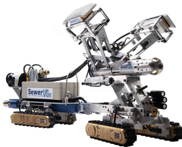
Figure 2: The SewerVUE Surveyor multi sensor inspection robot.
