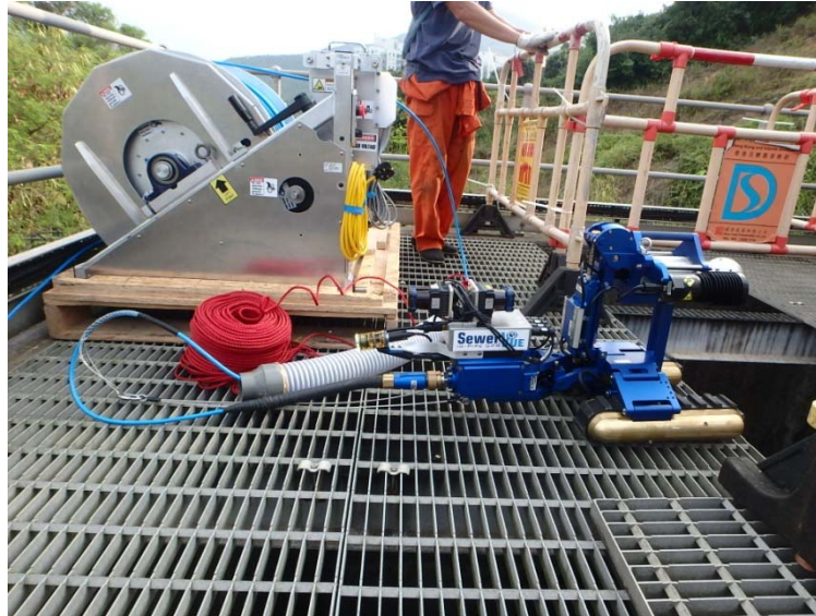
Figure 5. The multi-sensor inspection robot before deployment at Tolo Harbor, Hong Kong.
