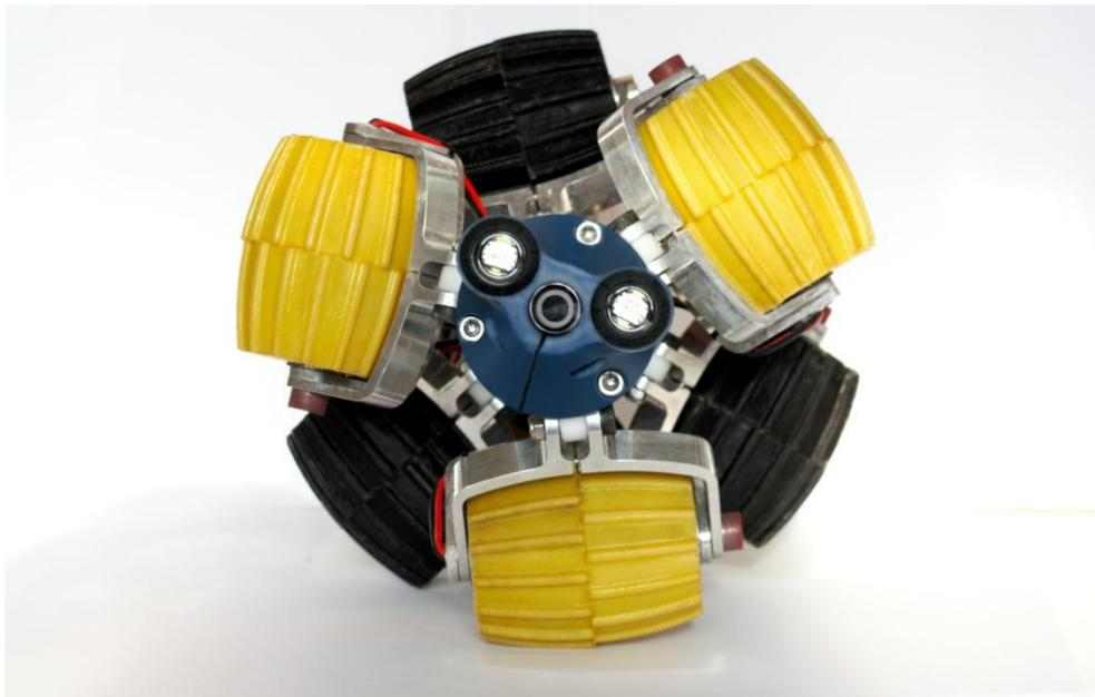
*Figure 2 – The Asbestos Cement Pipe Scanner.*
