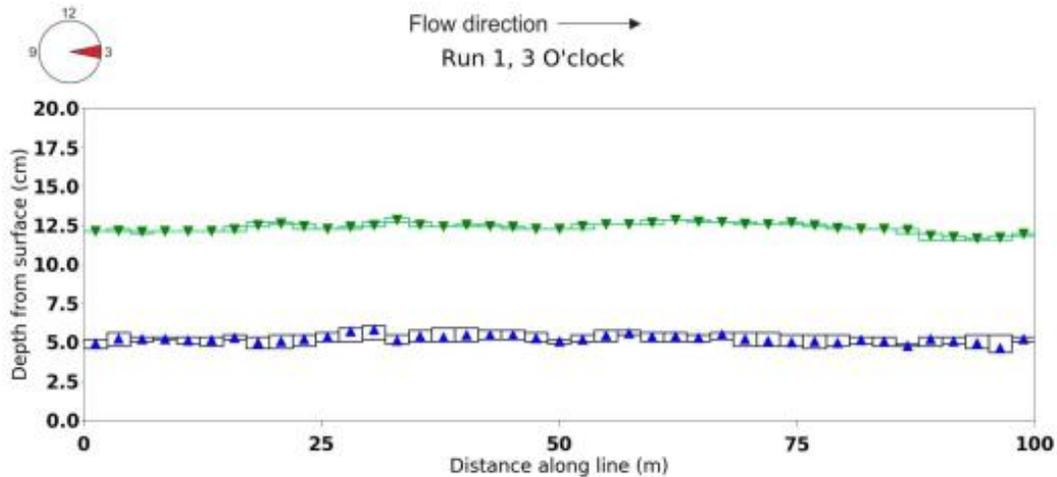
Figure 6 – PPR data from Mordialloc Main showing wall thickness (green line) and rebar cover (blue line).
