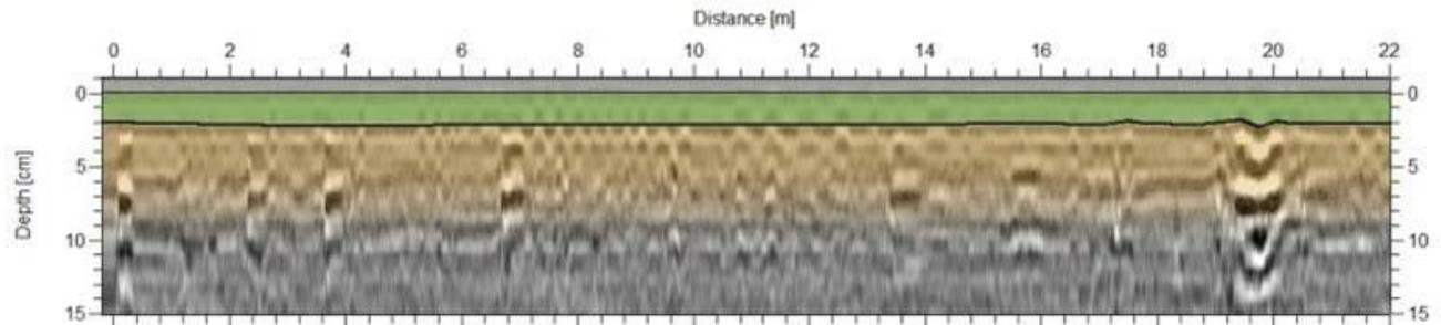
*Figure 4 – PPR data from the Harbourgreene Line. Wall thickness is represented by the green-shaded area.*
