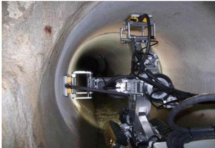
*Figure 1 – The Surveyor robot conducting a PPR survey of a concrete pipe.*
